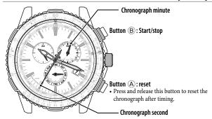
After 60 minutes of continuous chronograph operation, the chronograph automatically stops and is reset.
