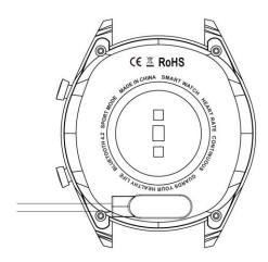
\* Note that the two contacts on the back of the watch cannot be in contact with each other with a conductor material or it will burn the circuit.
